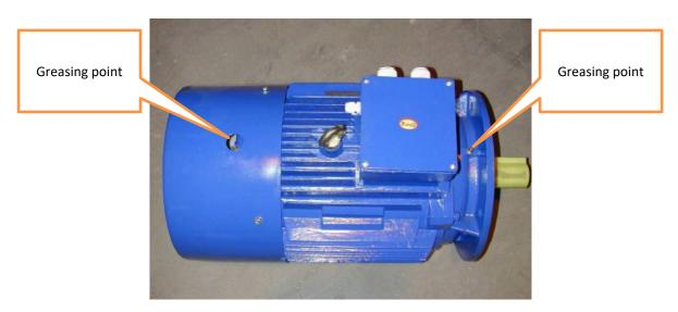
Figure 7-1 – Greasing point electric motors
