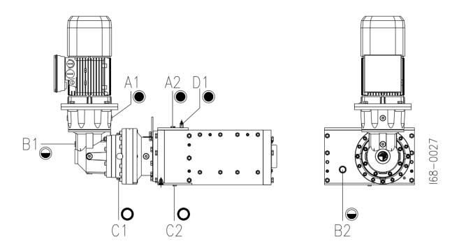
A= Oils filling plug, B= Oil Level indicators, C= Oil Draining taps, D= Grease filling plug
