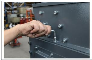
1. Remove the 6 M8 screws blocking the hopper.
