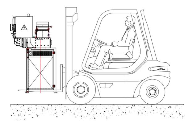
Figure 4-1 - Discharge from the machine
