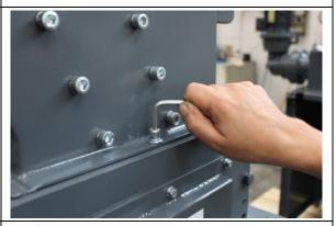
3. After the check close the cover hopper and tighten the hopper screws.
