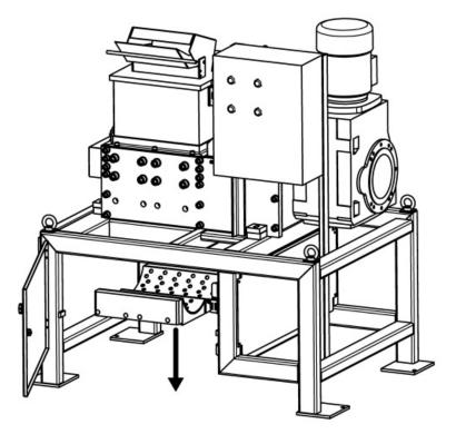
If the screen is stuck and will not slide down by gravity, you may use a crowbar (naildrawer / assembly lever) to pull it out of the chassis. attach it between the foot of the screen and the chassis of the machine and pull the screen down.
