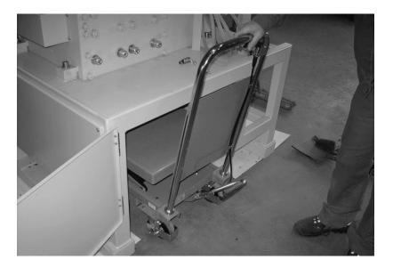
4. Loosen the bolts "B" (3 x silver allen bolts M16 each on front and 3 x silver allen bolts M16 on the rear of the cutting unit
