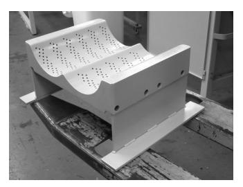
the chassis, so do not try to lift the screen any further, else you will lift the complete machine. Then the holes in the cutting block should match with the treads in the screen so that you can assemble the 4 large allen head bolts at the front and rear side of the cutting block. First tighten the 4 bolts at the front carefully, then the 4 bolts at the rear.
