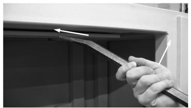
7. Once the screen is sitting on the platform lift, pull it out from under the shredder and remove all magnetic parts from accessible areas underneath the cutting knives and from the screen surface with suitable tools like heavy duty pliers. Also unblock the screen holes with a suitably sized punch. Be careful not to damage the screen
