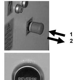
Please note that the hopper cover and doors at the machine are equipped with electric safeguards and must be closed during operation. Opening of door or hopper covers will immediately release an emergency-stop of the shredder. To re-start the machine, you need to close all doors and hopper covers and then restart the machine by pressing the green start-button.
