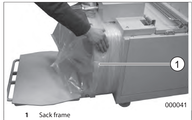
fig. 22 Installing a new plastic sack
