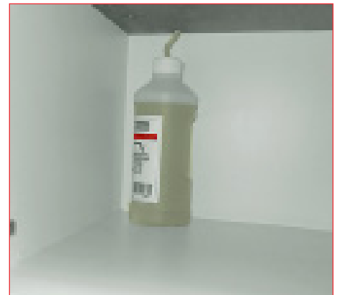
Built-in automatic oiler meters oil directly from plastic bottle - no reservoirs to refill
