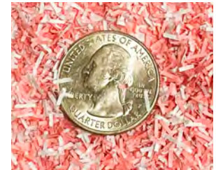
Actual 0.8 x 4.5 mm particles. 25% smaller than NSA requirements.
