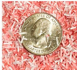
0.8 x 4.5 mm particles. 25% smaller than NSA requirements.
