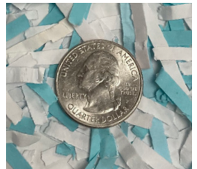
Example of particles created by intimus CP4 and CC3 shredder
